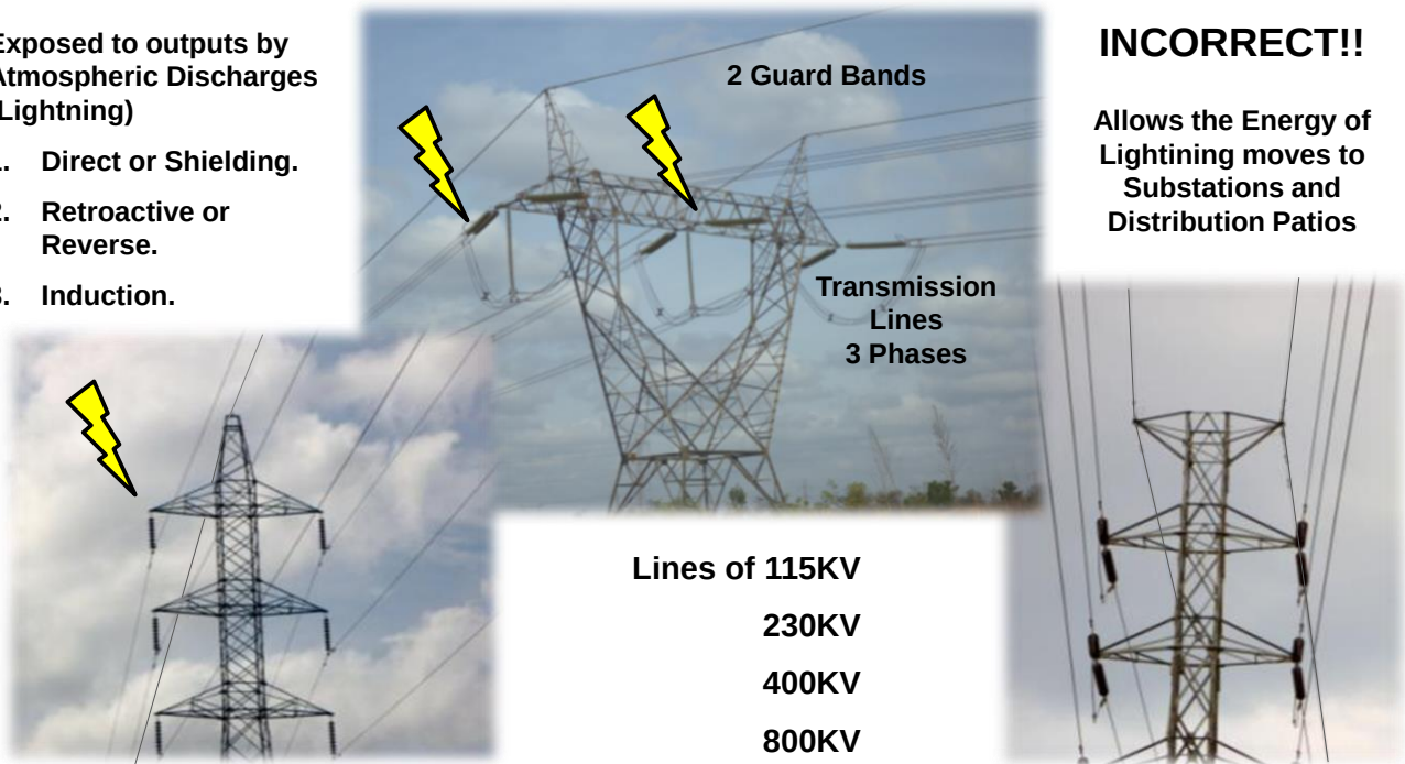
Picture 9. Guard Bands in different types of Towers and Transmission Lines.
